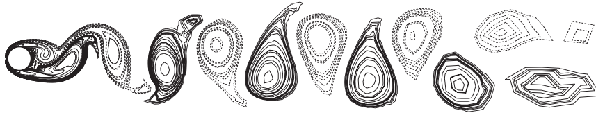
Figure 9. The vortex shedding captured behind the cylinder at Re=200 , test 1.
